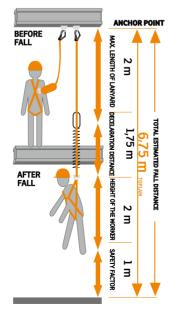
The energy absorber with lanyard is a component of personal fall arrest equipment and complies with EN355. Fall arrest system consisted of energy absorber with lanyard, attached to the full body harness (complied with EN 361) and connected to the structural anchor point (complied with EN 795) can be used as a basic personal protective equipment against falls from a height. Caution: The total length of the energy absorber with lanyard including terminations and connectors shall not exceed 2m.
